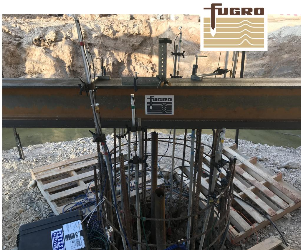
Testing under way with reference beam system to determine pile head movements.
